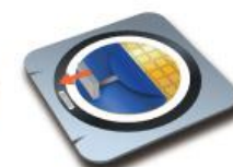
Removal of surface protective tape*
