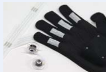
Wearable sensors using CNTs
