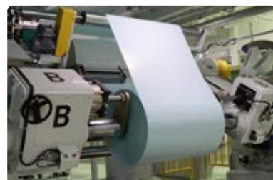
Coating equipment for solvent-less release paper (Kumagaya Plant)
